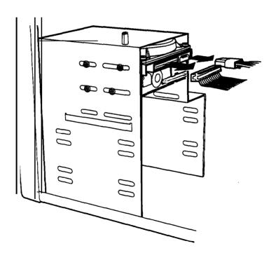
2. Remove the four screws securing the drive to the drive bay. There are two screws on each side of the drive.
